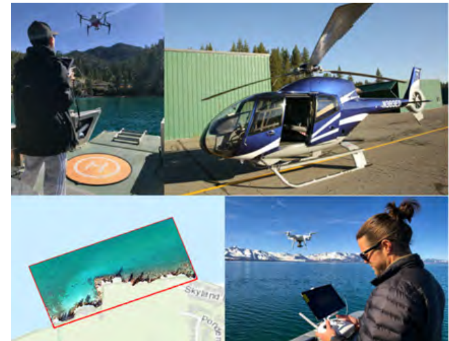
From top left, clockwise: Andy Wong launching a multispectral drone from R/V Bob Richards; cameras mounted on a helicopter; Brandon Berry completing a metaphyton drone survey; an orthomosaic image produced from the individual helicopter images.
