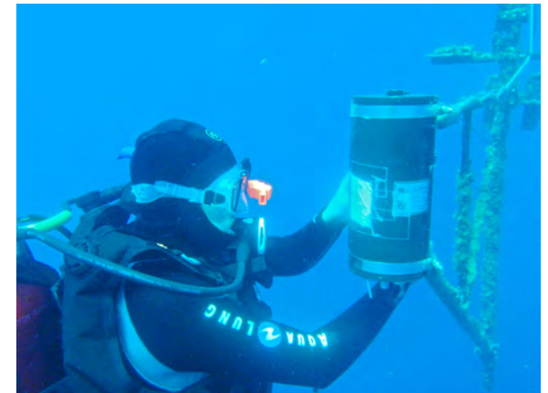
Cleaning the underwater radiometer at Buoy TB3, a joint project between TERC and NASA/JPL to continuously measure the changing light conditions in the lake.
