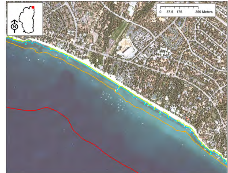
Four shoreline positions for Incline Village, NV. Green – the natural rim, blue- the 1992 drought, orange – a possible 5 year drought, and red – the ancient drought. Note the dock positions.
