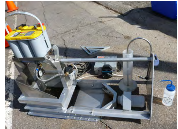
Wash-off simulator used to collect artificial stormwater samples. Photo: R. Townsend
