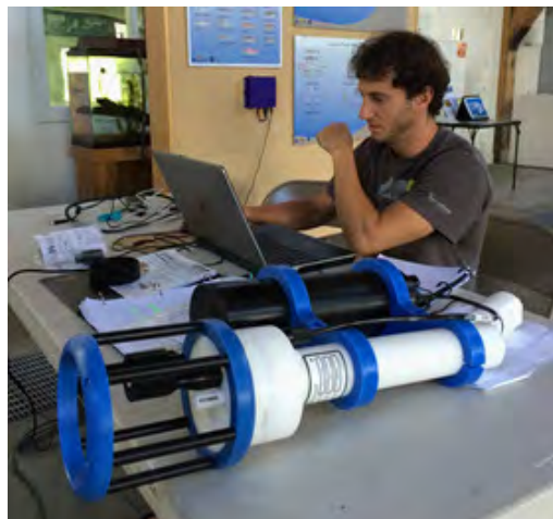
Graduate student Derek Roberts testing the RBR Maestro (white instrument) and the Turner C-3 (black instrument) Photo: G. Schladow
