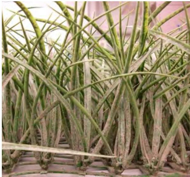
Synthetic plants in the experimental flume after an experiment. Accumulation of fine sediment is clearly evident. Photo: K. Fauria.
