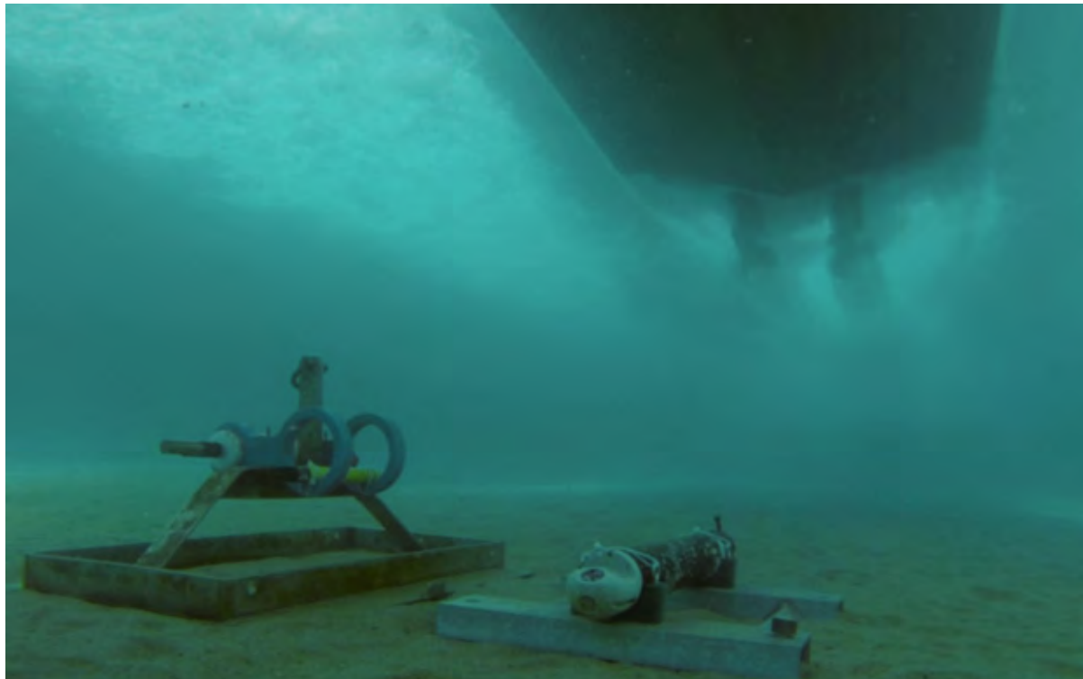
The instruments at Site C2 measuring water clarity (turbidity), pressure (depth), and water velocity induced by a boat travelling at 10mph over the site. Site R is out of the frame as it is 20 ft to the left of Site C. An in situ video camera was used for this image.
