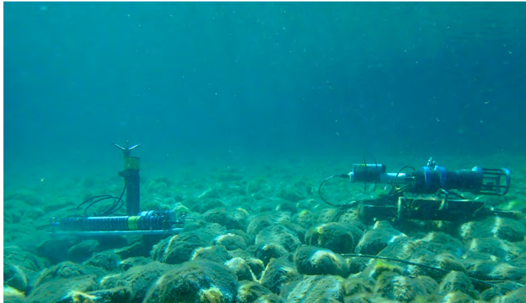
One of TERC's real-time Nearshore Water Quality Stations (right) with a newly installed Acoustic Doppler Anemometer (left) for turbulence measurements during UPWELL. The instruments were at 6.5 feet depth. Notice the heavy periphyton growth covering the rocks. Photo: B. Allen
