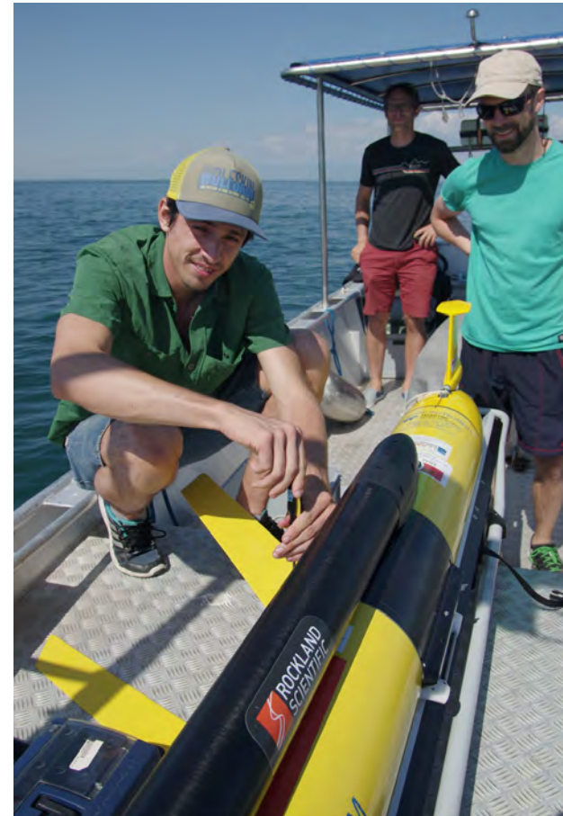
Oscar Sepúlveda mounting the microstructure package onto the glider at Lake Geneva. Photo: A. Bahr
