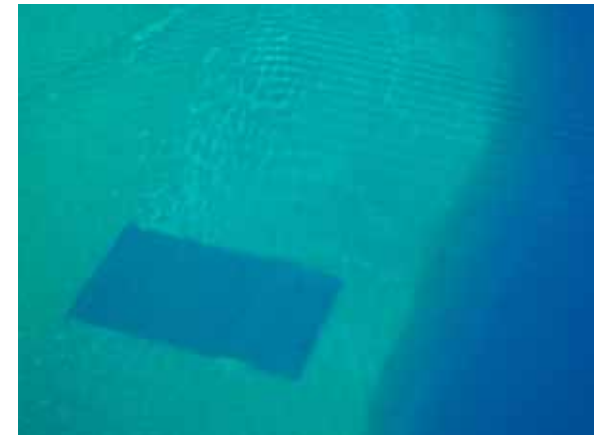
The large (one-half acre) bottom barrier deployed in Marla Bay is visible from the air
