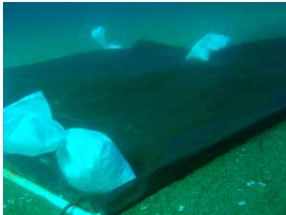
10-foot by 10-foot rubber bottom barriers were tested as a strategy for managing Asian clam populations
