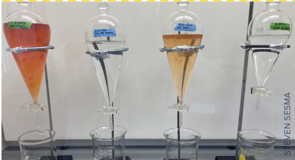
TERC chemist Steven Sesma places microplastics within a density separation funnel, where salt water allows microplastics to float to the top.
