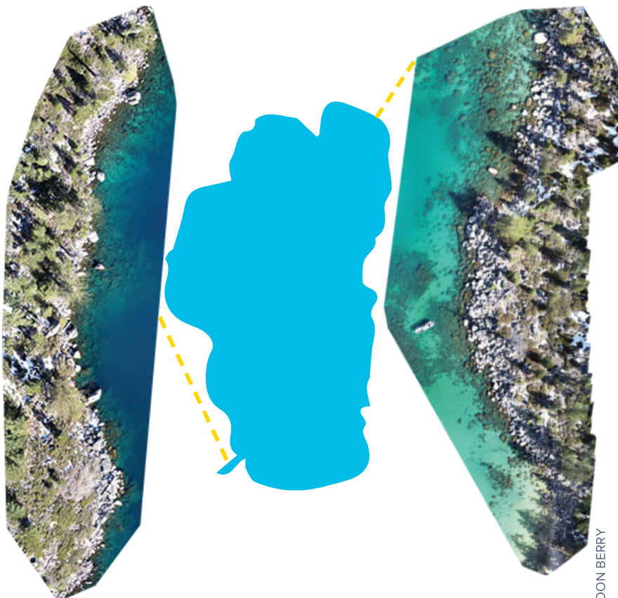
High resolution drone footage shows the shorelines of Rubicon (left) and Sand Point (right). These mosaics of drone images are used as a part of visual periphyton analysis.
