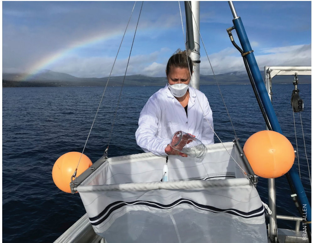
TERC researcher Katie Senft examines a manta trawl net, used to collect microplastic samples from the surface of Lake Tahoe.
