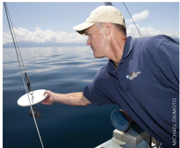
Recently retired TERC researcher Brant Allen prepares to take a Secchi depth measurement.
