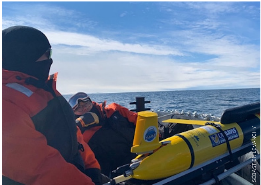
Drew Friedrichs and Seung-Tae Yoon in Terra Nova Bay deploying the Slocum glider Stormy, equipped with a Rockland Scientific MicroRider, from the R/V Araon's zodiac.
