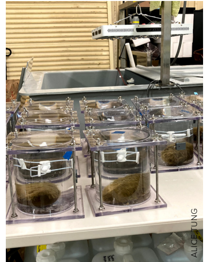
Scientists placed algae-covered rocks taken from the shores of Lake Tahoe into sealed plastic chambers to assess growth rates of the algae under controlled temperature and nutrient levels.
