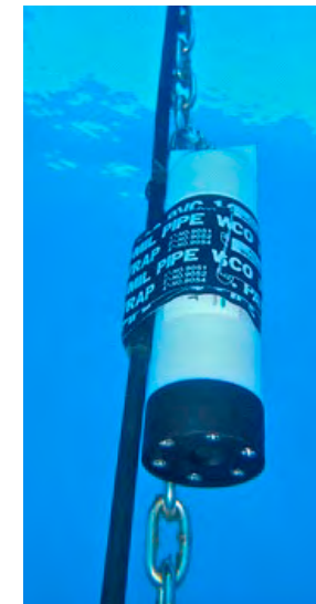
A dissolved oxygen sensor deployed in Lake Tahoe.
