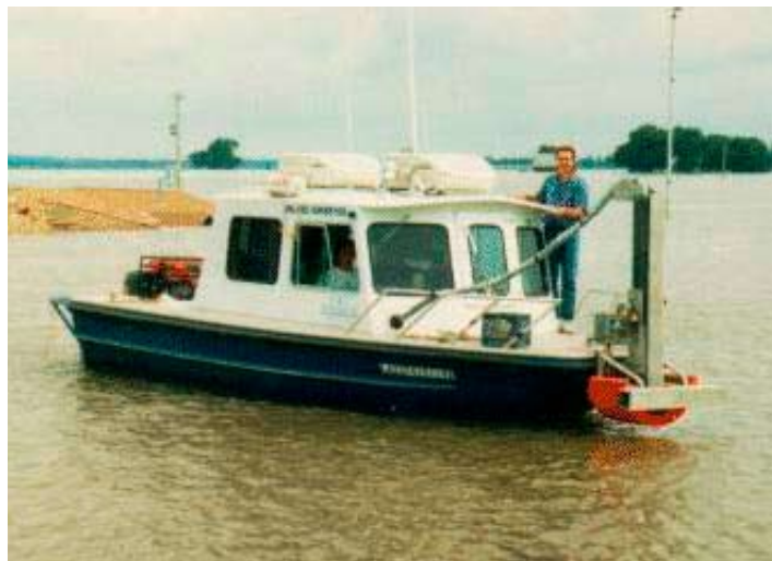
INLAND SURVEYOR WITH HIGH-RESOLUTION MARINE MULTIBEAM-SONAR MOUNTED ON BOW
