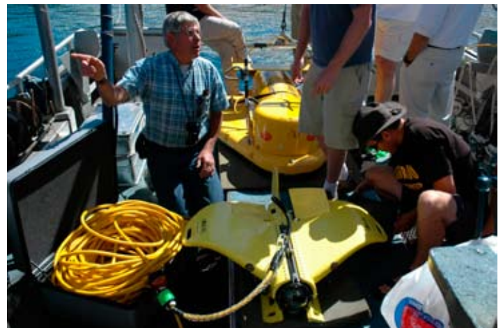
SCIENTISTS PREPARE TO LAUNCH THE HIGH-RESOLUTION SEISMIC CHIRP SONAR
