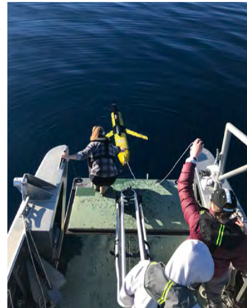
Launching the glider on its monitoring journey (left) and getting pulled from the lake after completing its Lake Tahoe mission (right). (Photos: B. Berry (left) and B. Allen (right))
