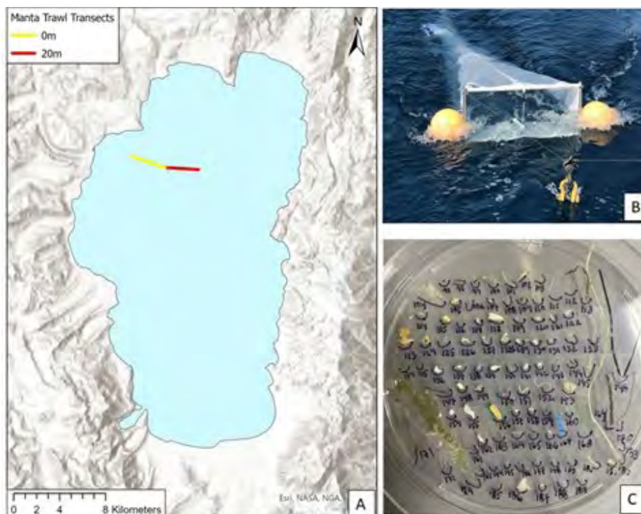
(A) Map of transect locations where microplastic samples were collected. (B) The manta trawl tow net. (C) Particles suspected to be plastic were isolated for subsequent Raman microspectroscopic analysis. (Photos: K. Senft (B) and S. Sesma (C))
