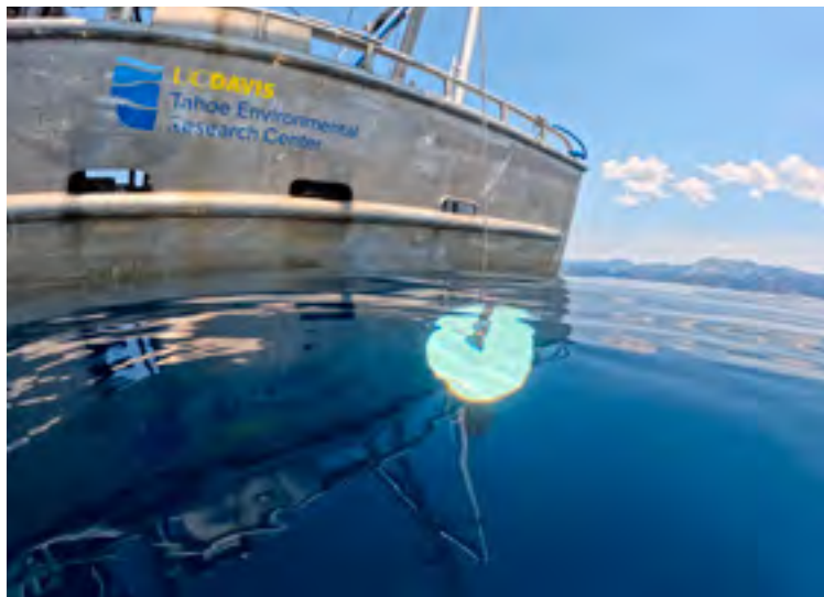
Figure 18. The Secchi disk begins its descent down the water column for a clarity reading (Brandon Berry, UC Davis TERC).
