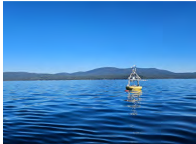
Figure 39. One of five buoys that calibrate NASA satellites and provide real-time data to the TERC Lake Conditions webpage (Alison Toy, UC Davis TERC).
