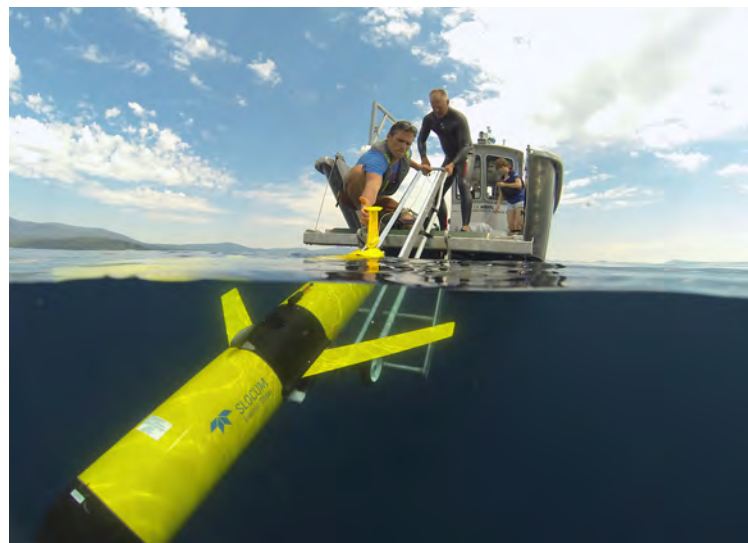
Alex Forrest deploys a glider in Lake Tahoe to facilitate research into turbidity, internal waves, and water movement around the lake. (UC Davis TERC)
