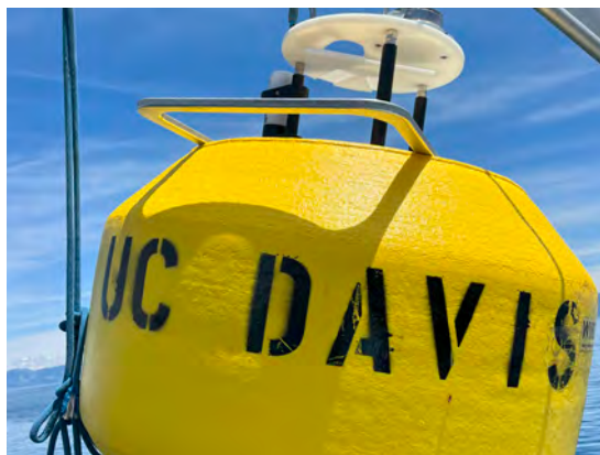
This buoy holds the Wirewalker in place. If you see it the lake, please do not touch, it is vital to take continuous measurements. (Keeler Nelsen, UC Davis TERC)
