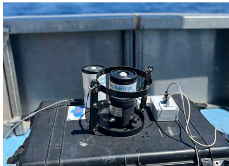
This multi-channel radiometer is used to capture UV penetration data by lowering it into Lake Tahoe during recurring monitoring trips in various locations around the lake. (Brandon Berry, UC Davis TERC)
