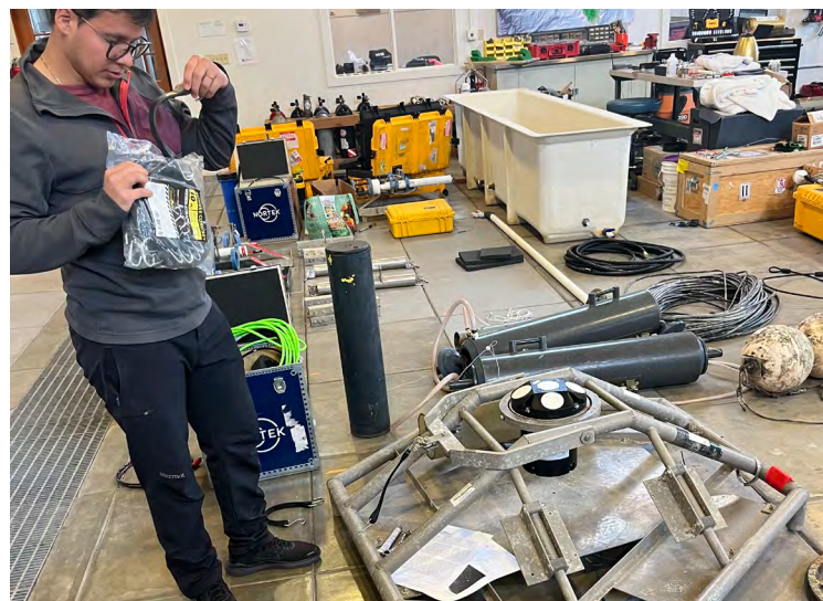
Sergio Valbuena works on metal frames that will hold the Acoustic Doppler Current Profilers (ADCPs) for their deployment on a recent project in Lake Tahoe. (Cara Hollis, UC Davis TERC)
