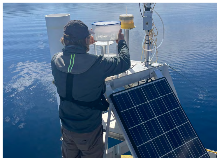
Michael Cane puts a new atmospheric deposition bucket on top of one of the four buoys permanently moored in Lake Tahoe. (Cara Hollis, UC Davis TERC)
