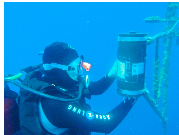
Cleaning the underwater radiometer at Buoy TB3, a joint project between TERC and NASA/JPL to continuously measure the changing light conditions in the lake.
