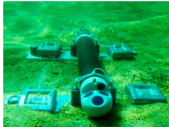
This Aquadopp instrument measured current velocity at one-inch intervals through the water column in Emerald Bay. The instrument was on loan from the University of Iceland.
