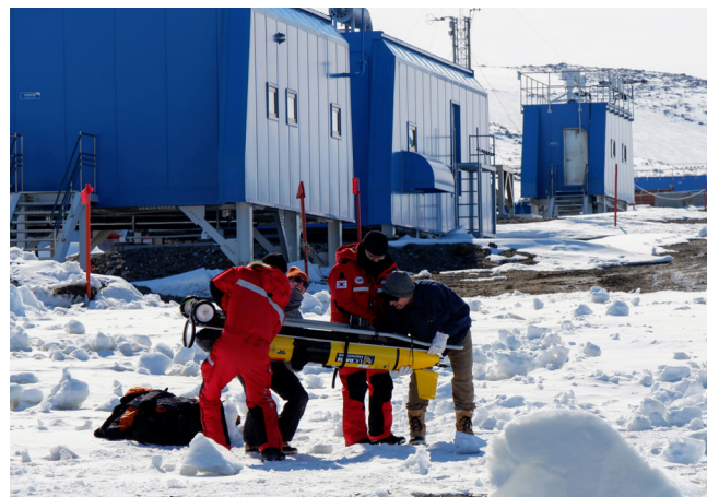
Calibrating the glider compass at Jang Bogo Station, Antarctica. Photo: J. McNerney
