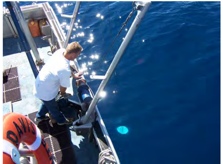
Boat captain Brant Allen measuring Secchi depth on Lake Tahoe
