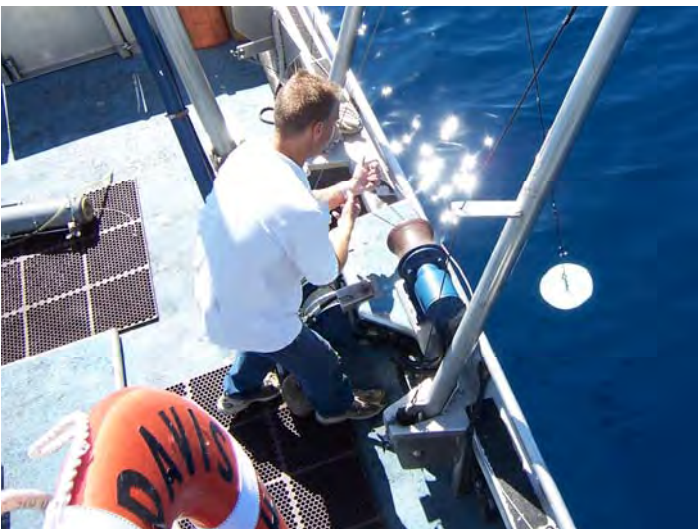
Boat captain Brant Allen measuring Secchi depth on Lake Tahoe
