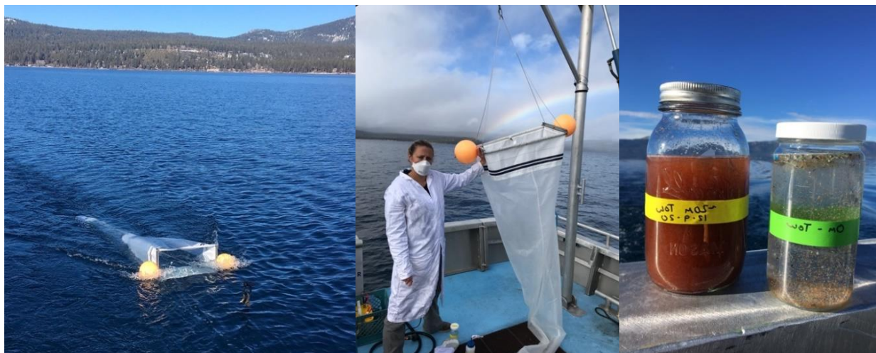
FIGURE 1. SAMPLING OF SUSPECTED PLASTIC PARTICLES FROM LAKE TAHOE SURFACE WATERS. A TOW NET WAS USED TO COLLECT SAMPLES FROM SURFACE AND SUBSURFACE WATERS (LEFT IMAGE). FOLLOWING A TOW, ALL MATERIAL FROM THE NET WAS TRANSFERRED INTO A SAMPLING JAR (MIDDLE IMAGE). SAMPLES FROM EACH JAR WERE PROCESSED AT THE LAB TO REMOVE ORGANIC MATERIAL AND ISOLATE ANY POTENTIALLY PLASTIC PARTICLES FOR FURTHER ANALYSIS.
