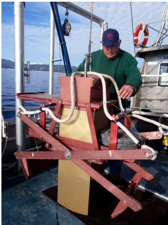
FIGURE 4. BOX CORE SAMPLER PREPARING TO BE DEPLOYED DURING SEDIMENT SAMPLING ON LAKE TAHOE
