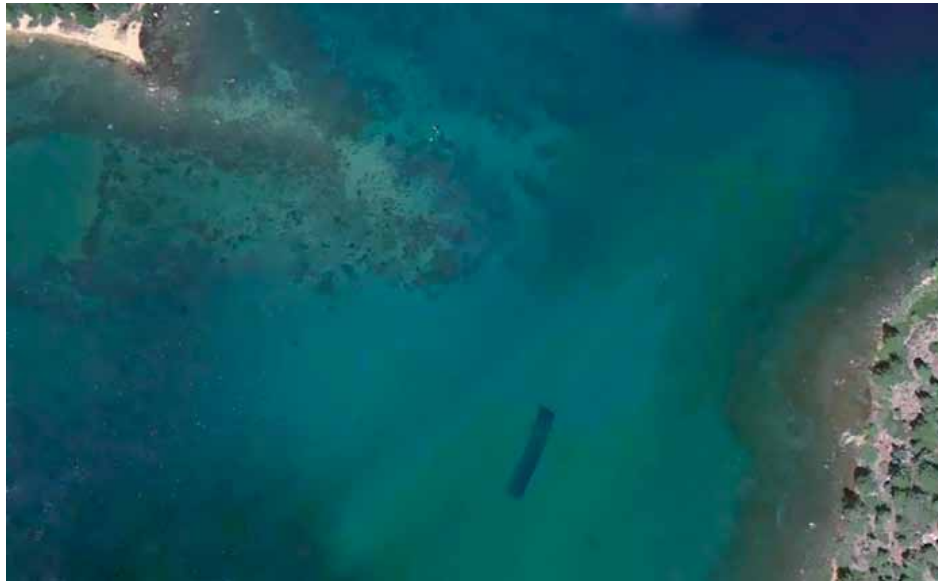
Aerial photo of the rubber bottom barrier installed on the sill of Emerald Bay
