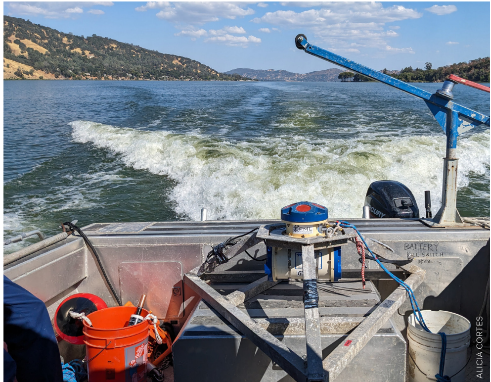
Acoustic Doppler Current Profiler (ADCP) used to measure currents in Clear Lake and to evaluate exchange between the three basins of this lake.
