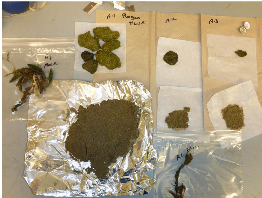
Figure 23 . Example of metaphyton samples from Regan Beach on shore, on 9/21/15, separated into sand and various organic and inorganic fractions. Separated algae fractions are on 3 pieces of white weighing paper at the top (Regan shoreline sites “Left” A-1, “Center” A-2, and “Right” A-3. Separated sand fractions for each site are below on foil (A-1) and two white weighing. Pieces of aquatic plants and clamshells were also separated from the metaphyton collected.
