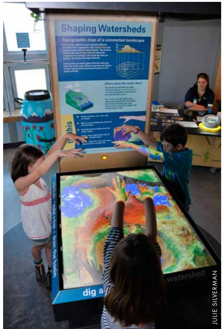
The Interactive Sandbox captivates young and old visitors alike with evolving color contours that reflect the sculpted sand surface, and water flow simulations show the passage of floods through the created watershed.
