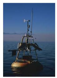
A mini-vol on TERC buoy collects data from the Angora Fire. Smoke can be seen behind the buoy.
