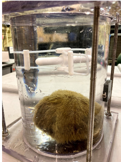
Sealed periphyton incubation chambers were used to measure growth.
