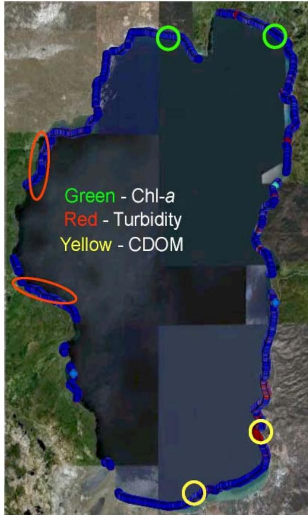
Figure 25. Detail of Lake Tahoe showing results of the optical backscatter channels with areas of relatively high intensity of each component (chlorophyll-*a*, turbidity and CDOM) at the 5 m lake contour.
